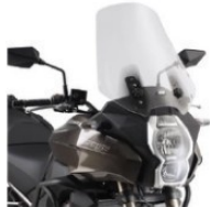
D4113ST 5,800-. Specific screen, transparent, 53 x 45 cm (H x W) to be mounted instead of the original screen
